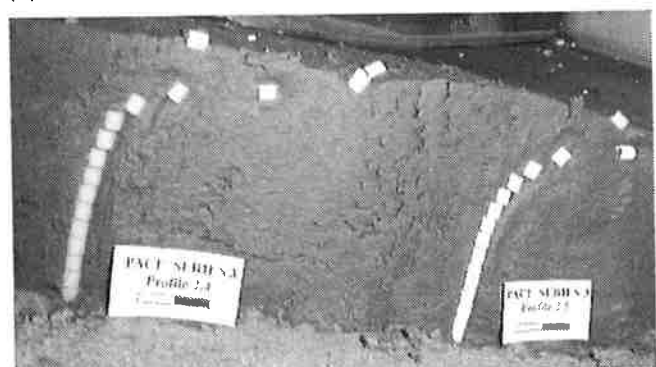
Figure 1. Soil displacement profiles (a) 12° slope, four cycles of freeze-thaw; (b) 18° slope, two cycles of freeze-thaw.
