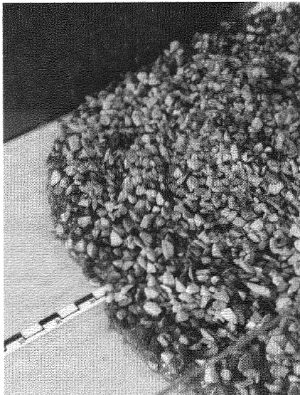
Figure 2. Slightly mixed mass comprised of sand and gravel heterogeneously covered by a brittle layer of dry gravel: Distinctive ridges appear, single gravel particles are dislocated, viscous material is pushed from underneath to the surface and amplitude of ridges increases (exp. no 18).
