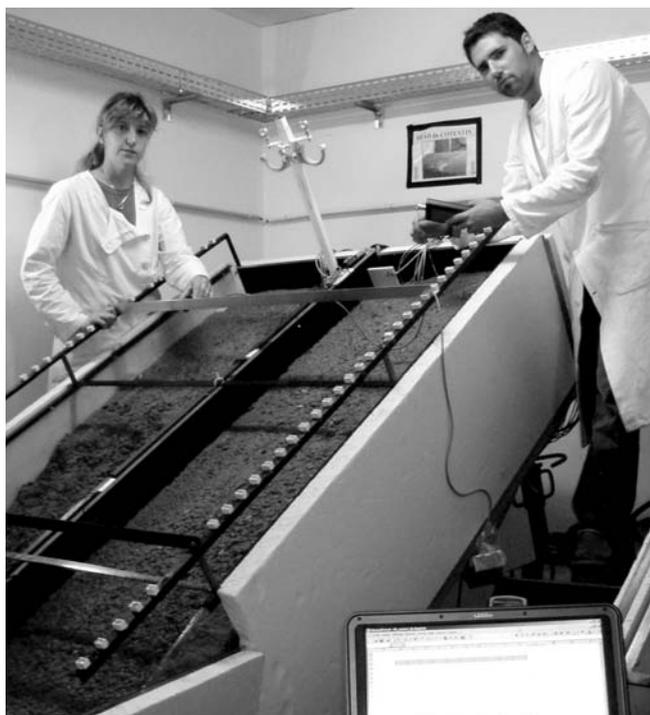
Physical modelling of slope morphology during climate warming at Caen laboratory. Photograph by G. Guillemet.
