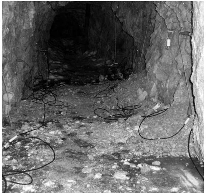
Geophysical monitoring of rock permafrost in a gallery near Zugspitze North Face (Germany/Austria) at 2770 m asl. Photograph by M. Krautblatter.
