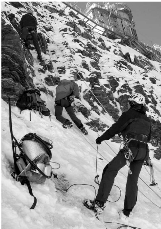
Installation of a PERMASENSE wireless sensor network in an ice face on the northern side of Sphinx/Jungfrauojoch (3500 m asl). Photograph by S. Gruber.
