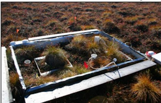
Carbon exchange is monitored during the growing season with automated chambers, and  $^{13}\text{C}$  and  $^{14}\text{C}$  are used to partition respiration fluxes into contributions from autotrophic, heterotrophic, young and old soil C. In order to better understand the mechanisms responsible for changes in C dynamics we also measure thaw depth, water table depth, plant growth and community composition, NDVI, plant phenology, plant tissue nitrogen (N) content and soil N cycling.
