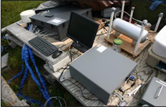
*Measuring  $\delta^{13}\text{C}$  of ecosystem respiration using the Picarro G2121-i*
