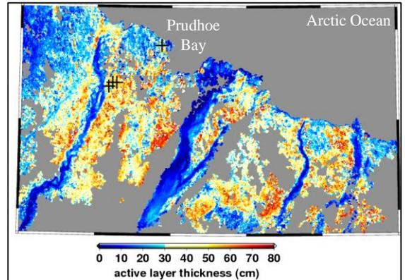
1992-2000 average Remotely Sensed Active Layer Thickness (ReSALT) for the Prudhoe Bay area on the North Slope of Alaska derived from the European Remote-Sensing Satellite (Liu et al., 2012).
