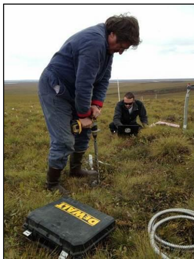
Vladimir Romanovsky (GIPL Group Leader) drilling a hole in the ground to install temperature sensors and Bill Cable preparing the sensors for installation at a permafrost observation station on North Slope of Alaska (Photo: Santosh Panda).
